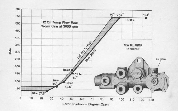
The new oil pump has been used on and after Engine H2E-16078. The reduced oil flow, and better gas consumption provide the H2 with greater range and performance.
