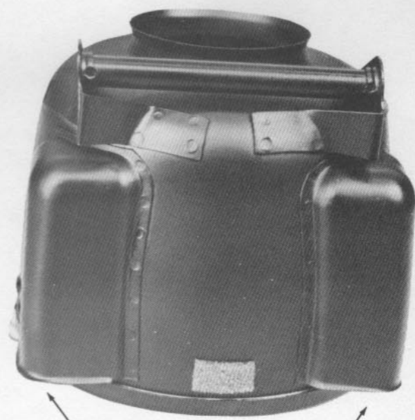
ADDITIONAL AIR INTAKES
