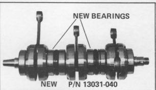
To improve lubrication of the two new bearings, additional oil passages have been bored into the upper crankcase half. These cases have been installed on all S2's from engine number S2E-24749 up. The part number is unchanged.
