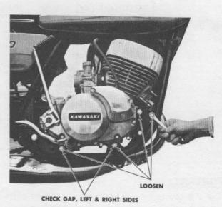
B. Without removing the engine, use a thickness gauge to check the clearances between the engine bosses and the frame lugs on both sides of the engine.
