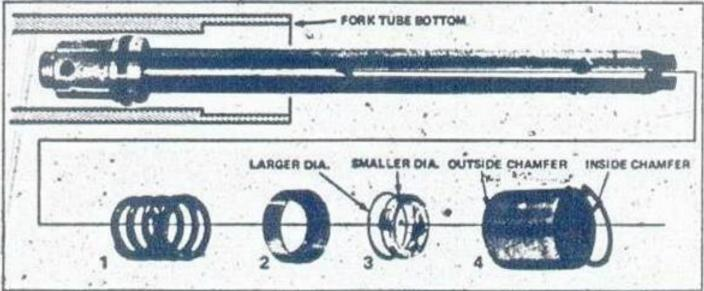
Install the snap ring carefully into the fork tube to hold the pieces securely in place. Steps for completing fork assembly are outlined in the Shop Manuals.
