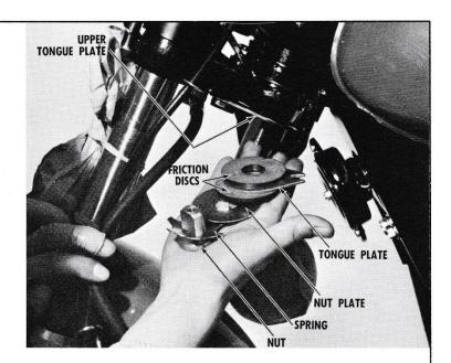
The upper tongue plate is bolted to the lower triple clamp at the factory. Install the parts shown in the previous step, taking care to engage the tongue plate with the frame stud. Screw the nut, with spring, onto the damper shaft. Finally, insert the safety cotter pin and split the ends.
