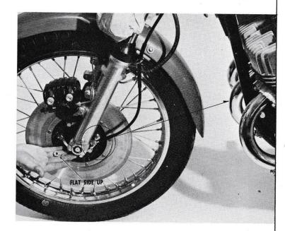
Tighten the axle mounting caps securely. Take care to keep the gaps equal, as shown.
