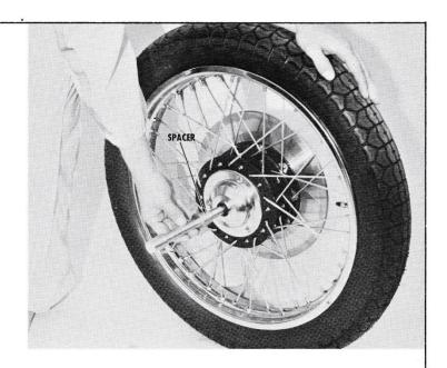
Tighten the axle securely. Then turn the speed-ometer drive assembly to check for binding.
