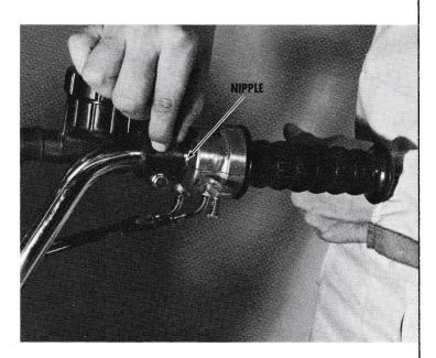
Turn the adjuster and thumbwheel into the lever holder as far as possible and then back them out until the slots line up. Push the cable nipple up into the lever socket. Pull on the cable sheath, and then swing the cable into the adjuster and release it.
