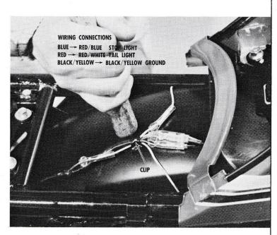
Install the seat assembly with the hinge pins, as shown. Be sure to install the safety clips.
