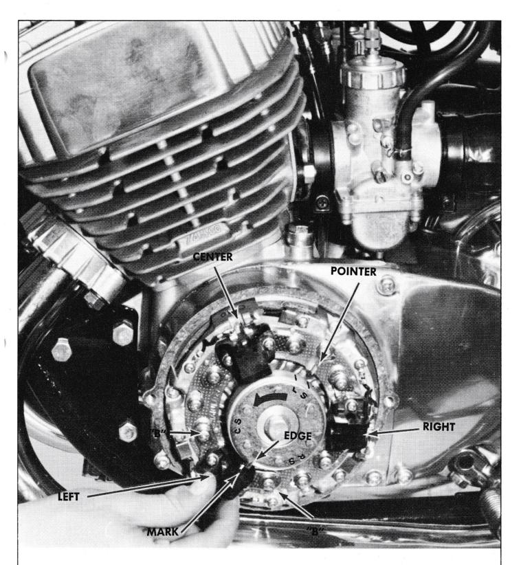
Turn the crankshaft in the direction shown until the "S" (static) mark nearest the "L" mark lines up with the pointer. The trailing edge of the rotor tab should align with the mark on the pick-up for the left-hand cylinder, as shown. If it does not loosen the two screws "B" and adjust the pick-up accordingly. Tighten the screws securely after adjustment.
