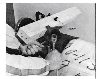
Remove the four handlebar clamp bolts and lockwashers, and discard the plate and hold-down bolt. Temporarily, reinsert the handlebar clamp bolts with lockwashers.
