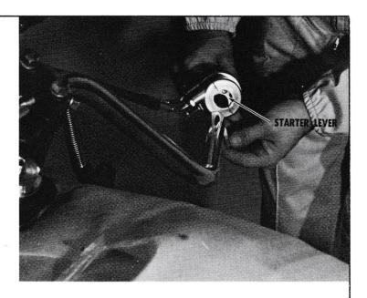
Mount the brake master cylinder next to the twistgrip. The nipple on the side of the handlebar clamp cap is to space the master cylinder assembly the proper distance from the twistgrip. Tighten the bolts to about 4.5 lb.-ft. of torque.
