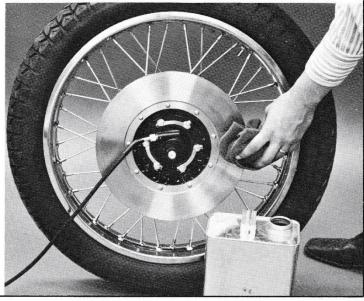
Remove the cardboard spacer from between the caliper pads. Lift the front wheel into position with the disc between the caliper pads, and the axle ends between the axle mounting studs.
