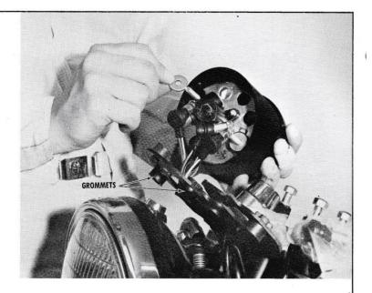
Check to be sure that the rubber lens shade at the top of the meter fits into the metal housing all around. Fit a thin washer and an acorn nut to each stud and tighten them securely.
