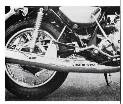
Turn on the main switch and operate the front and and rear brakes individually. The front brake light switch does not require adjustment. The brake light should turn on when the rear brake pedal travels %". Adjust the brake lamp switch by loosening the locknut and turning the adjusting nut. Tighten the locknut after adjustment.
