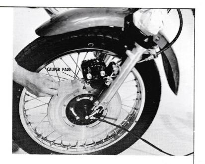
Fit the axle mounting caps with nuts and lock-washers, but do not tighten them yet.
