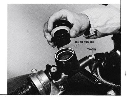
Check to be sure both banjo bolts on the three-way fitting are tightened to 20 lb.-ft. of torque. The brakelight switch should be tightened to 13 lb.-ft. of torque.
