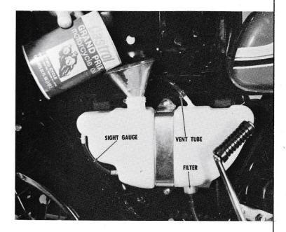
Check to see that the chain oiler hoses are clear and firmly attached to the oiler valve, and that the lower hose is routed through the hole on the top of the chain case cover. Remove the oiler tank cap and fill the tank with 5 fl. oz. of good quality SAE 30 motor oil.
