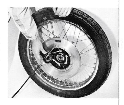
Insert the axle spacer into the hub grease seal, as shown, and thread in the axle.
