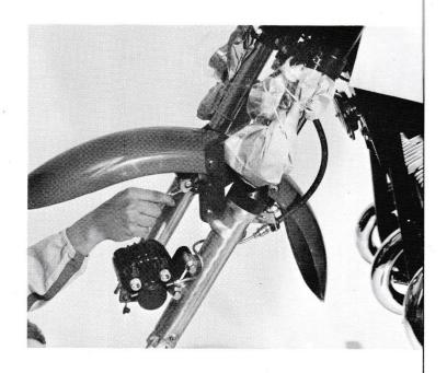
Check the inside of the speedometer drive gear assembly for loose parts and fit it to the front wheel hub. Be sure to align the tangs in the drive assembly to the recesses in the hub.
