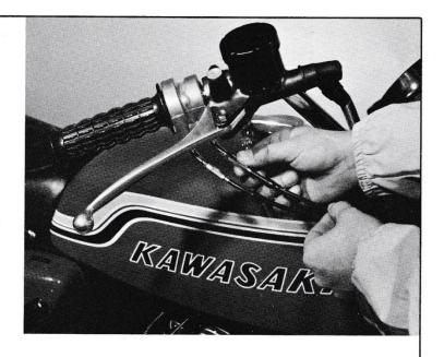
Tug on the starter cables to check for free play, which should be 1/8" in each cable. NOTE: If there is no slack, the starter plunger will be held open slightly, causing rich mixtures from the carburetor. To adjust the cable slack, pull up the rubber cap, loosen the locknut, and turn the adjuster. Tighten the locknut after adjusting.
