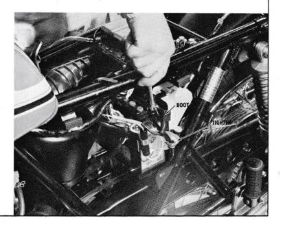
Connect the black ground wire to the negative (—) battery post. Check to be sure that the ground screw on the frame is tight.
