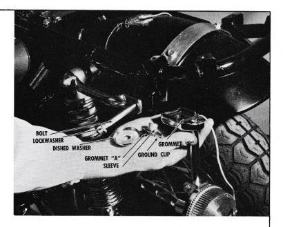
Tighten the bolt securely, and plug the wire from the left turn signal lamp into the green lead, and the wire from the right turn signal lamp into the gray lead.
