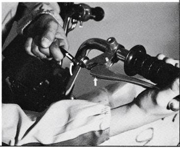
Mount the left-hand grip case with the wiring harness on the bottom and tighten the two Phillips head screws. Fit the two handlebar wiring straps, as shown.
