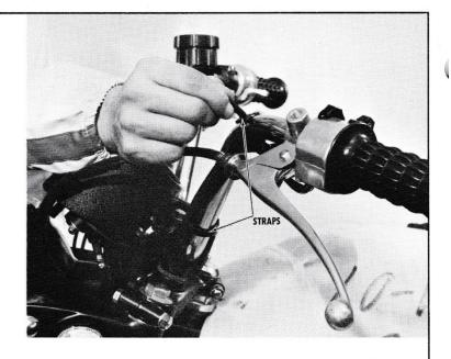
Mount the rear view mirror on the clutch lever holder. Tighten the locknut when the mirror is in the proper position, and strip off the protective plastic backing. Insert the plug in the other mirror mounting hole. Finally, remove the protective packaging material from the fuel tank.
