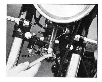
Check to be sure these hydraulic fittings are tightened to about 12.5 lb.-ft. of torque. The bleeder valve should be tightened to about 6.5 lb.-ft. of torque.
