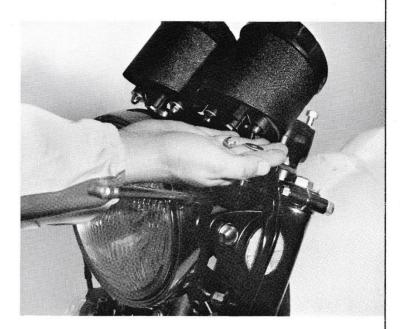
Route the speedometer cable through the bracket on the lower fork tube, through the loop on the lower triple clamp, inside the headlight bracket, and into the cable socket. Spin the front wheel slowly to ease the insertion of the cable into the socket. Slip the tachometer cable into its socket, and tighten both ring nuts securely.
