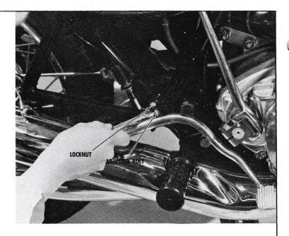
The rear brake pedal must have  $\frac{1}{2}$ " to  $\frac{1}{2}$ " of free movement. If it doesn't, turn the adjuster nut accordingly.
