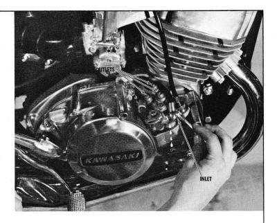
Start the engine and maintain a steady engine speed of 1500 to 2000 rpm. Hold the oil pump control lever in the wide-open position to bleed any air out of the oil pump body and oil pressure lines. When the exhaust starts to smoke heavily, release the lever and stop the engine. CAUTION: If the exhaust does not smoke, or if bubbles are present in the oil pressure lines, check for blockage or loose connections.
