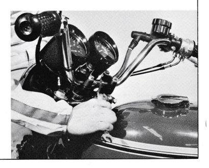
Stack the steering damper parts, as shown here, before installation. CAUTION: Clean off any oil or grease with an oilless solvent, such as trichloroethylene, to insure smooth damper action. Follow these assembly instructions exactly to prevent steering difficulties.
