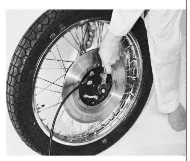
Wipe the disc clean with trichloroethylene or other oilless solvent.
