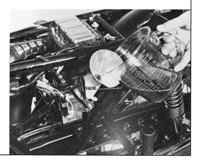
Remove the oil pump cover. Loosen the oil inlet banjo bolt to bleed the oil inlet line from the oil tank. After two minutes of oil flow, tighten the bolt. CAUTION: If the oil flow is slow or stops altogether, check the oil tank filter for clogging and the oil hose for pinching. Check to be sure that the three oil outlet bolts are tight.
