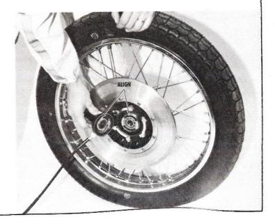
Insert the axle spacer into the hub grease seal, as shown, and thread in the axle.
