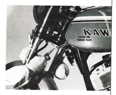
Mount the front turn signals. All the necessary hardware is already "strung" on the turn signal lamp wire in the proper order of assembly. Be sure the face of the lens is vertical during the final tightening.
