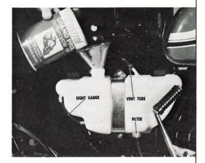
Check to see that the chain oiler hoses are clear and firmly attached to the oiler valve, and that the lower hose is routed through the hole on the top of the chain case cover. Remove the oiler tank cap and fill the tank with 5 fl. oz. of good quality SAE 30 motor oil.
