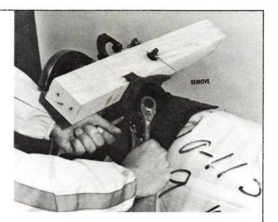
Remove the four handlebar clamp bolts and lockwashers, and discard the plate and hold-down bolt. Temporarily, reinsert the handlebar clamp bolts with lockwashers.
