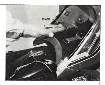
Make the wiring connections as shown, and then slip all the wires from the rear turn signals and the taillight under the clip on the fender. Bend the clip down to hold the wires in place.
