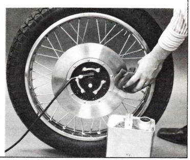
Remove the cardboard spacer from between the caliper pads. Lift the front wheel into position with the disc between the caliper pads, and the axle ends between the axle mounting studs.
