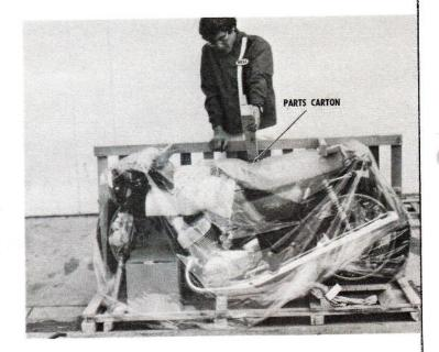
Lift out the front wheel assembly, the two parts cartons, and the dual seat assembly, and remove the handlebar by prying loose the strap holding it to the base of the crate. With an assistant, move the motorcycle to the work area and park it on its center stand.
