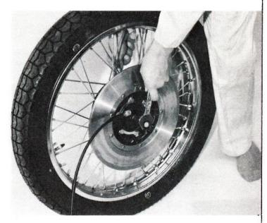
Wipe the disc clean with trichloroethylene or other oilless solvent.
