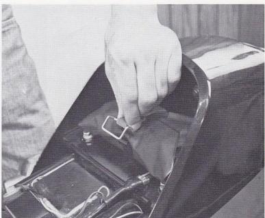
Mount the passenger grab rail by slipping the front of the rail between the flatwashers on the upper shock mounts, and screwing the two mount bolts into the rear mounting lugs from under the seat backrest.
