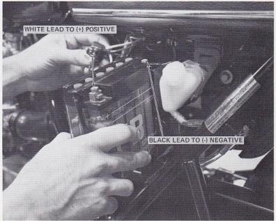
Secure the battery in place with the bracket, and position the fuse in the clip. Route the vent hose through the guide, behind the battery box, and through the rubber guide on the fender. This will insure that the vent is not pinched or allowed to drain on the chain or other critical points.
