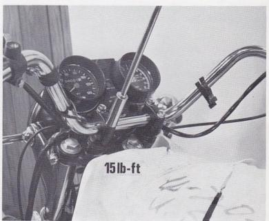
Tighten the two clamp screws on the twistgrip assembly. **NOTE:** make sure the rubber grip does not rub on the end of the bar.
