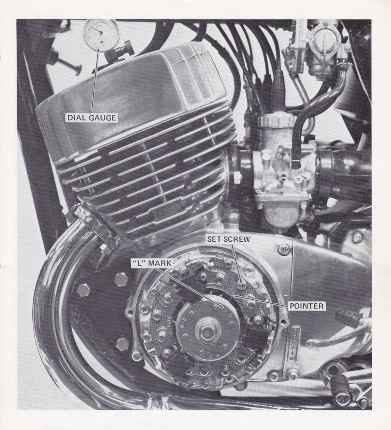
Remove the spark plug and fit a dial gauge to the left cylinder. Turn the crankshaft to top dead center and then rotate it clockwise until the dial gauge shows that the piston is 3.13mm BTDC. The pointer should
