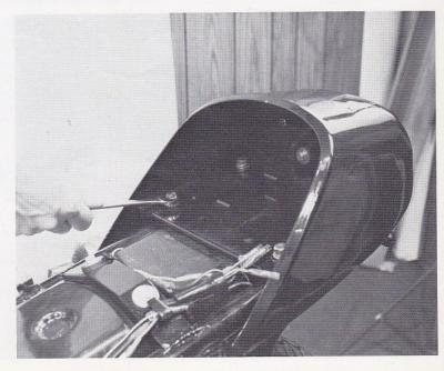
Make the wiring connections as shown, and then slip all the wires from the rear turn signals and taillight under the clip on the fender. Bend the clip down to hold the wires in place.
