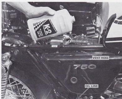
Remove the oil pump cover. Loosen the oil inlet banjo bolt to bleed the oil inlet line from the oil tank. After two minutes of oil flow, tighten the bolt. CAUTION: If the oil flow is slow or stops altogether, check the oil tank filter for clogging and the oil hose for pinching. Check to be sure that the four oil outlet bolts are tight.
