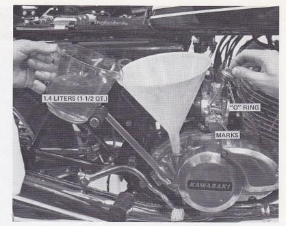
Check the oil line from the oil tank to the pump to make sure it is secure, and check the oil tank vent hose to make sure it is not pinched or blocked, which could result in serious engine damage. Fill the oil tank with a good quality 2-stroke oil, such as Kawasaki K-2.
