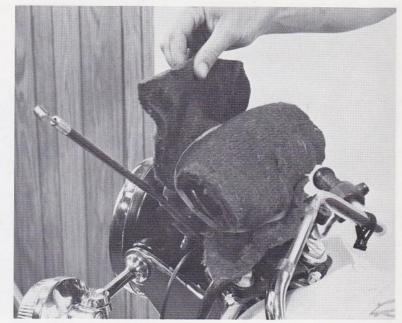
Mount the handlebars and tighten the clamp bolts to 15 lb.-ft. of torque.
