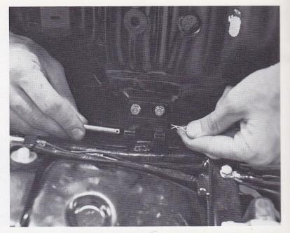
Attach the seat stop rod by slipping the short end with the washer through the slot in the frame crossmember. Attach the top end to the seat with a cotter pin.
