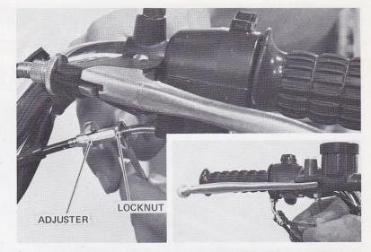
Tug on the starter cables to check for free play, which should be 1/8" in each cable. **NOTE**: If there is no slack, the starter plunger will be held open slightly, causing rich mixtures from the carburetor. To adjust the cable slack, pull up the rubber cap, loosen the locknut, and turn the adjuster. Tighten the locknut after adjusting.
