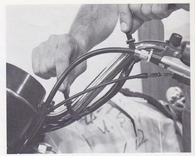
Mount the rear view mirror by threading it in all the way, backing it out to the proper position, and tightening the locknut securely. Also put the mirror mount plug in the socket on the brake lever bracket.
