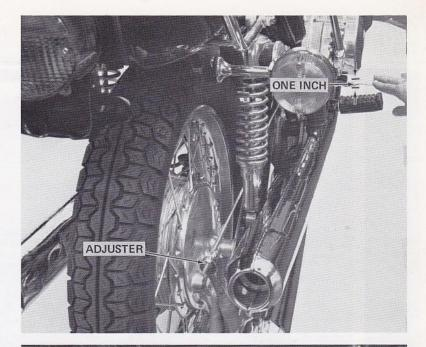
Turn on the main switch. The brake lamp should light when the brake pedal is depressed 1/2" to 3/4". If it does not, loosen the adjuster nuts and adjust the switch as required. Test the front brake lamp switch, the head light, high and low beam, the taillight, the turn signals, and the horn.
