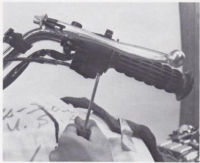
Turn the clutch lever thumbwheel and adjuster as far into the lever bracket as possible and then back them out until the slots align. Push the nylon-protected cable nipple into the socket on the lever, pull on the cable sheath, and swing the cable into the adjuster.
