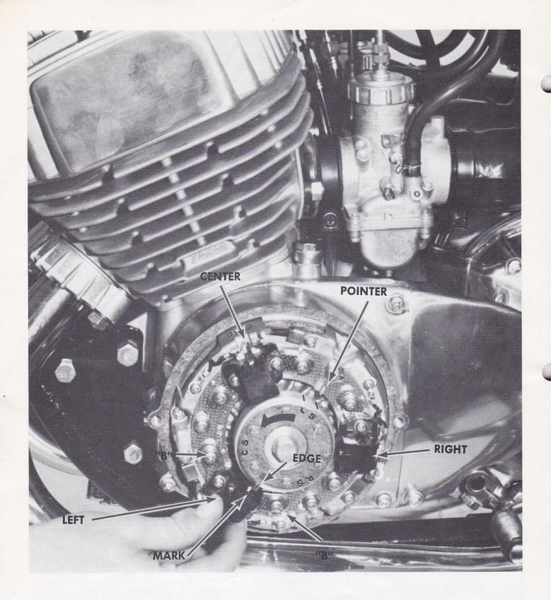
Turn the crankshaft in the direction shown until the "S" (static) mark nearest the "L" mark lines up with the pointer. The trailing edge of the rotor tab should align with the mark on the pick-up for the left-hand cylinder, as shown. If it does not loosen the two screws "B" and adjust the pick-up accordingly. Tighten the screws securely after adjustment. Turn
