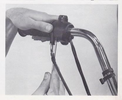
Mount the front brake master cylinder next to the twistgrip. The small nipple on the side of the clamp spaces the master cylinder the proper distance from the grip assembly. Tighten the bolts to 4.5 lb.-ft. of torque.
