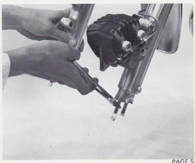
Slip the cardboard spacer from between the brake pads and fit the front wheel to the unit. The disc should slide between the pads of the brake caliper, and the axle should rest between the axle clamp studs.
