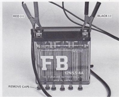
Wash off any spilled acid with fresh water. Be sure the battery damper rubber is in place to protect the battery. Before sliding the battery into the box, connect the black lead to the negative terminal. Then slide the battery into the box with the vent tube facing out. Connect the white lead to the positive terminal (+).
