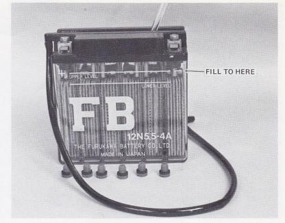
To avoid battery damage when charging, remove all of the caps. Connect the battery charger leads (red to +, black to -) to the battery posts. **CAUTION:** Do not charge at a rate greater than 1 amp. Charge for 15 to 20 hours. Discontinue charging if the electrolyte temperature rises to 115°F. If the electrolyte level drops, refill the battery with **distilled water only!**
