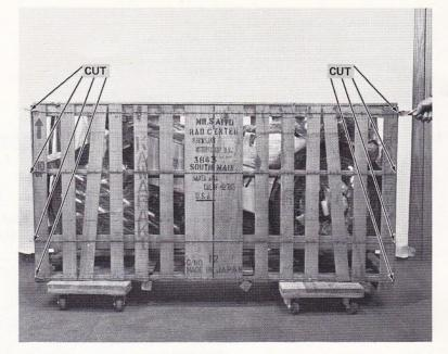
On the wooden crate, pry off the top of the crate and fold down the ends and one side; or lift the cardboard cover straight up off the foam crate. **CAUTION**: Peen over all nails to prevent injury or a tire puncture.
