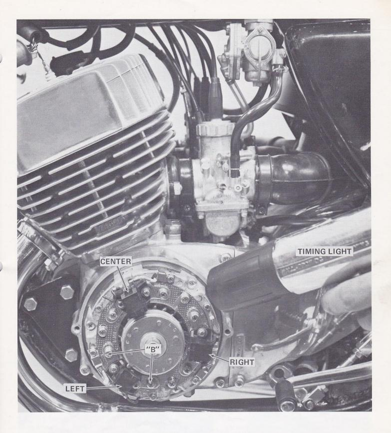
Connect a stroboscopic timing light to the left-hand sparkplug wire. Start the engine and maintain a steady speed of 4000 rpm. Using the timing light, check to see that the pointer aligns with the "L" mark on the rotor. If it does not align, loosen the two
