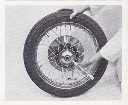
Tighten the axle to 55 lb.-ft. of torque, then turn the speedometer drive gearbox to check for binding.
