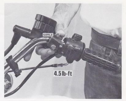
Mount the left-hand switch case between the grip and the clutch lever so that the cold start lever and the headlight beam control are easily reached. Tighten the screws securely.
