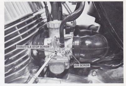
Finally, lengthen the cable adjuster at the twistgrip so that there is approximately 1/16"-1/8" play in the throttle. Do the same to the starter cable.
