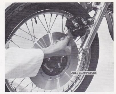
Mount the axle clamp caps, as shown, so there is no gap in front, and an even gap at the rear. Align the yellow point marks on the fork and axle to correctly position the speedometer drive gearbox. Then tighten the front nut of the left axle clamp, then the rear nut to 14 lb.-ft. of torque. Depress the forks several times to center the axle, and then tighten the right axle clamp nuts, front then rear, to 14 lb.-ft. of torque.
