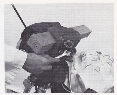
Remove the nut holding the wooden crossbrace and discard the brace. Then remove the handlebar clamp bolts.
