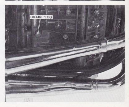
Fill the transmission with 1.4 liters (48 oz.) of SAE 10W-40, 20W-50, or 10W-50 motor oil marked SD or SE. The oil level should be between the two marks on the filler cap dipstick. Be sure the O-ring is in place.
