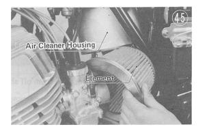
The air cleaner housing of the H1 cannot be removed without first unmounting the left carburetor.
