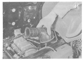
Unscrew the air duct clamp at the bottom of the air cleaner. Remove the air cleaner mounting screw.
