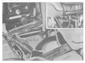
Push the air ducts forward (or take them off altogether) and pull out the air cleaner.
