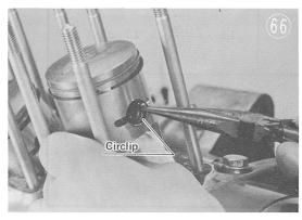
Remove each piston by pushing its piston pin out the side that snap ring was removed. Use the piston pin puller and adapter "A" (special tools) if necessary.
