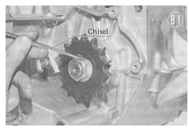
Hold the sprocket with a sprocket holder (special tool) to remove the sprocket nut, and then remove the sprocket.
