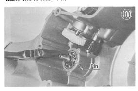
CAUTION: Do not remove the oil seal unless it is damaged.
