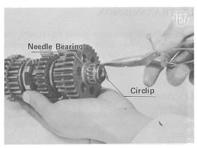
Remove the oil seals and bearings.
