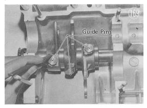
Pull out the shift drum and remove the selector forks.
