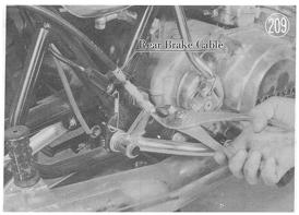
Take off the lock nut, pull out the pivot shaft and remove the swing arm.
