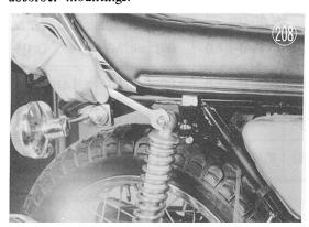
Unhook the brake lamp switch spring, and on the H1 also remove the rear brake cable.
