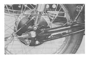
To make reassembly easy, loosen the chain adjuster lock nut and back off the adjuster screw 2 or 3 turns.
