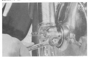
Place a stand under the engine to raise the front wheel off the ground. Unscrew the axle, and remove the wheel and brake panel as an assembly.
