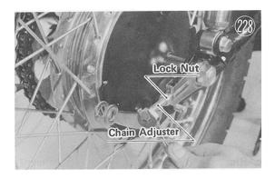
Pull out the cotter pin and take out the axle The right chain adjuster collar will come off at the same time.
