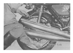
Loosen the axle nut and loosen both chain adjusters. Push the rear wheel forward to slip the chain off the sprocket, and pull the chain up over the chain guard out of the way. The wheel can now be pulled off together with the sprocket.
