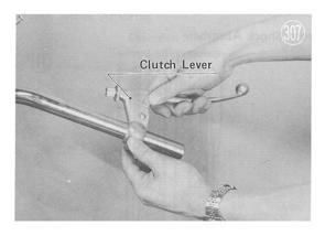
Unbolt the upper half of the left mounting and remove the handlebar.
