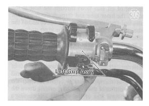
Remove the clutch and brake lever assembly.
