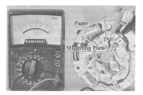
(2) Check the contact points for wear or fouling. The points must be inspected periodically since they become worn after a long period of operation, and the slight sparking at each break gradually burns the surface.
